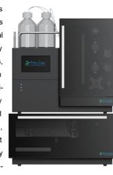
junction with fully automatic combustion instruments to achieve direct sample injection (solid, liquid) and high-temperature pyrolysis for the determination of halogens and sulfur. They can also be used in conjunction with ICPMS for elemental speciation analysis.
