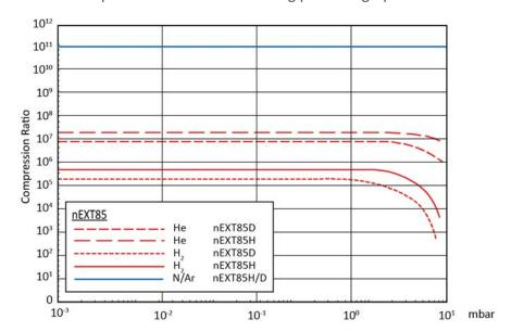
Figure 15 nEXT85 compression ratio versus backing pressure graph
