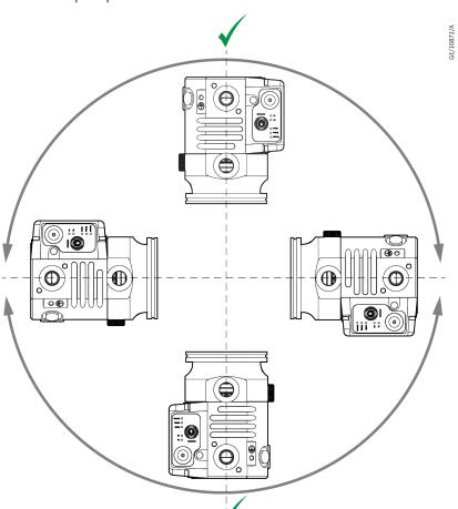
Figure 19 Allowable pump orientation
