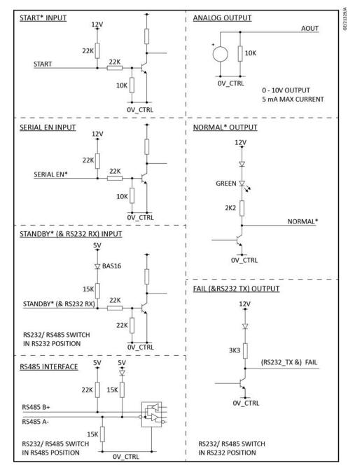
Figure 12 Interface circuits for nEXT turbo pump controllers
