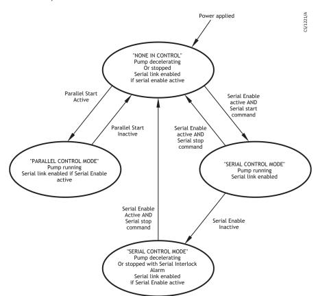
Figure 28 Serial and parallel control flowchart
