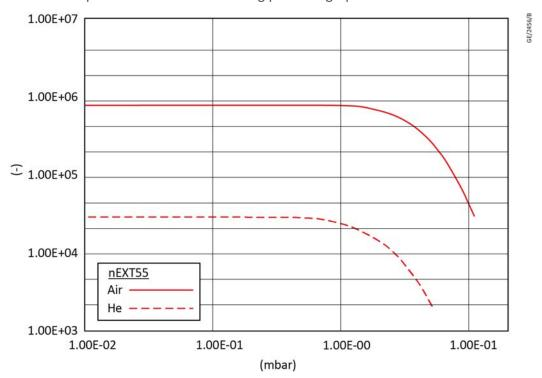
Figure 17 nEXT55 compression ratio versus backing pressure graph
