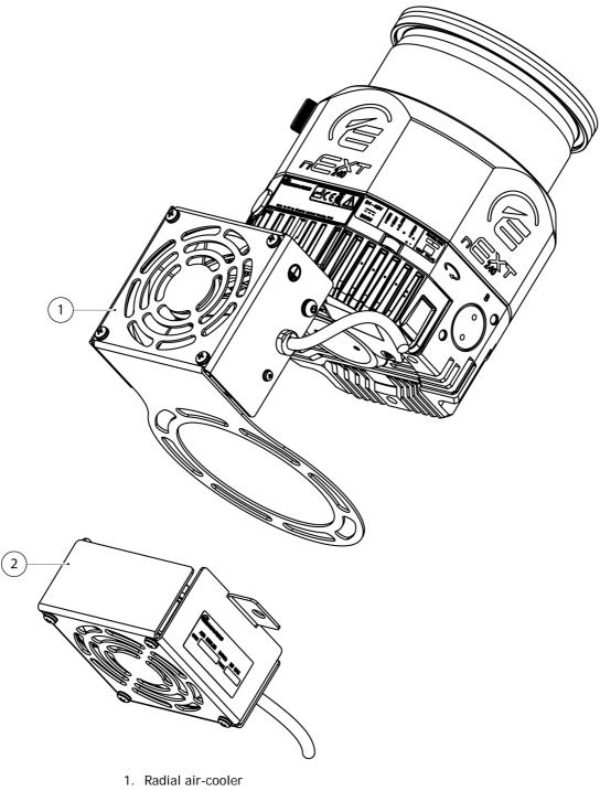
Figure 7 - ACX nEXT radial and axial air cooler installation
